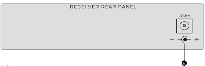
Stand-alone Power supply Connector: DC5V 2A Input
